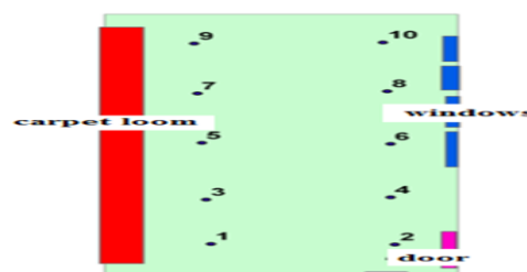
Fig. 2: Positions of measurement stations (1–10), carpet looms, windows, and doors in workshop II.
