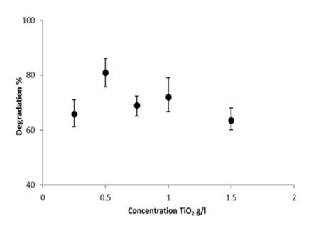
**Fig. 1:** The Effect of  $TiO_2$  concentration (0.25- 1.5 g/l) on the Methyl Orange degradation (19.77 mg/l).
