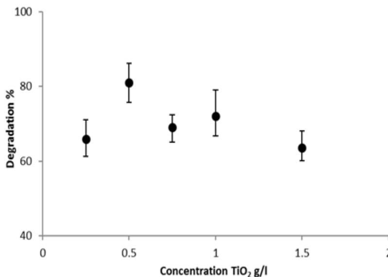
**Fig. 1:** The Effect of TiO<sub>2</sub> concentration (0.25- 1.5 g/l) on the Methyl Orange degradation (19.77 mg/l).
