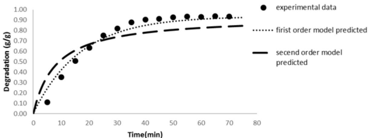
**Fig. 3:** The non-Linear plots for the pseudo-first and second order kinetic model for the methyl orange degradation.
