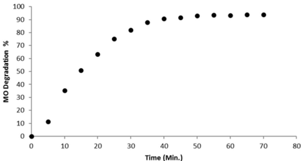
**Fig. 2:** The Effect of photocatalytic reaction time on Degradation efficiency of Methyl Orange (MO).
