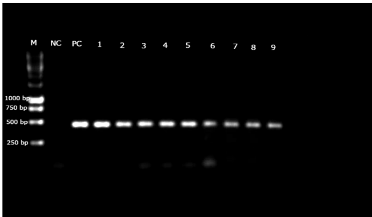
Fig. 3: The Gel electrophoresis of the PCR products of Acanthamoeba spp. isolated from the water samples of Zanzan province, Iran. Lane M: standard DNA marker (250 bp), lane NC: negative control, lane PC: positive control and the lanes 1 to 9 are representative of the water Acanthamoeba isolates.
